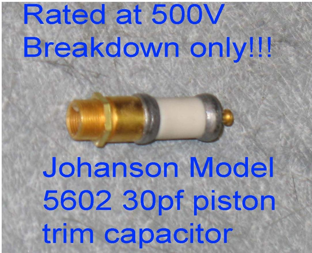
It turns out the capacitor manufacturer is still in business and I was able to obtain replacements direct from the Johanson Manufacturing . The part number designation is 5602 air capacitor. Cost was 21.44 a piece as of March 2008.
