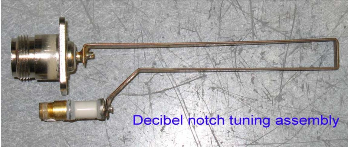
It is easy to unsolder the capacitor with the notch tuning assembly removed.
