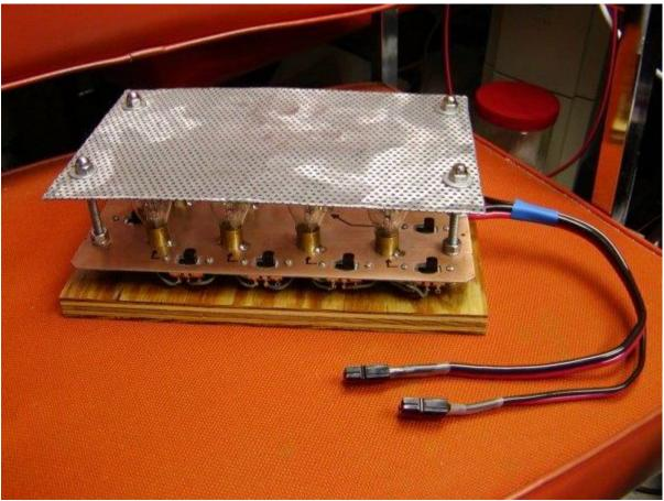
This is a simple load bank constructed using 12 automotive tail lamps #1157. They are wired such that the low current (tail light) filaments which draw 600 ma each are connected through one side of DPDT switchs to a power buss brought out on one of the Power Pole connectors. The high current (brake light) filaments which draw 2.1 Amps each are connected through the other side of the DPDT switchs to a separate power buss which is brought out on the other Power Pole connector on larger wire.
