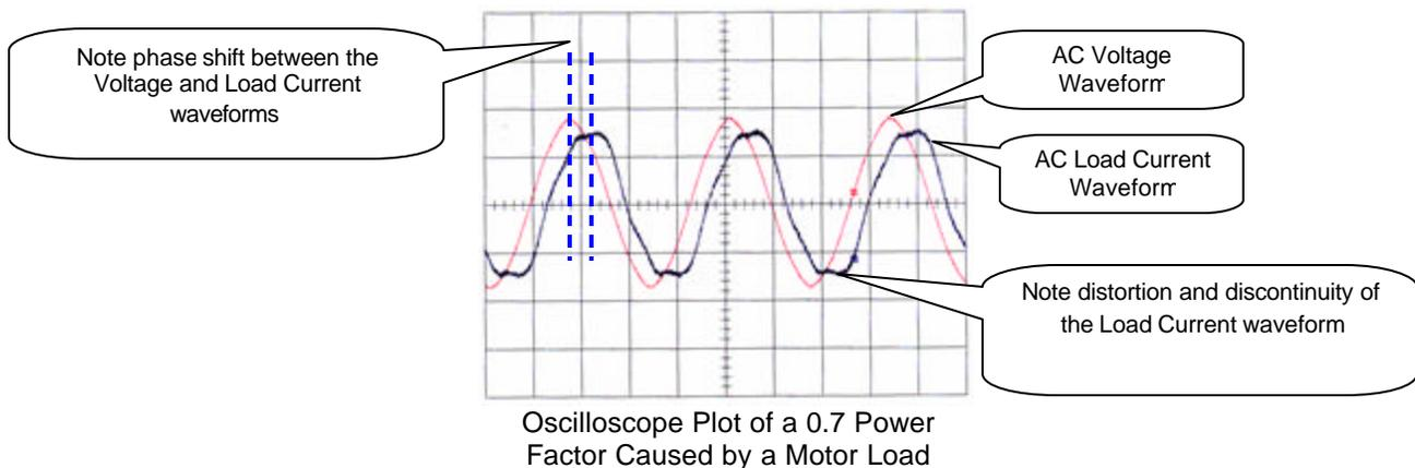
A distorted Load Current waveform can be the result of a non-linear load such as a rectifier, variable speed drive, discharge lighting, or a switching power supply typically found in most computers and sophisticated electronic equipment.
