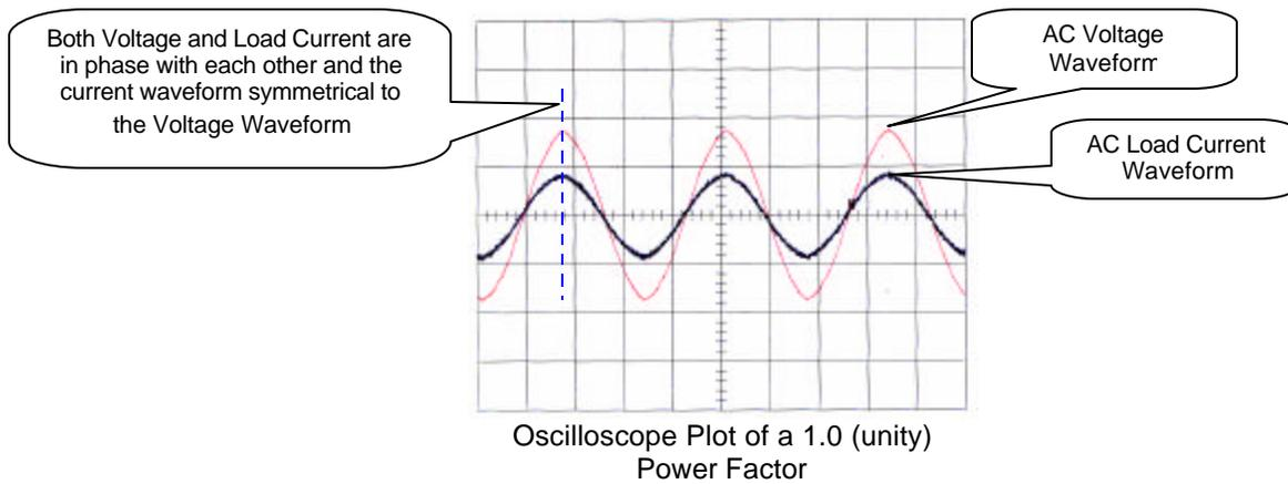
A poor power factor can be the result of either a significant phase difference between the AC Voltage and AC Current measured at the load, or can be due to a high harmonic content or a distorted/discontinuous load current waveform.
