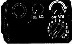
TURN POWER ON by turning the Volume knob clockwise past the OFF detent.
