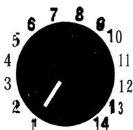
The Channel Selector knob has 14 positions. The Radio has 28 channels which are separated into two "groups" of 14 channels each. Group 01 is factory programmed for narrow channel (12.5 kHz) FM reception. Channel Group 02 is programmed for wide channel (25 kHz) FM reception. Use Group 02 for proper communication with the original AN/PRC-127 Radio.
