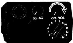
**TURN POWER ON** by turning the Volume knob clockwise past the OFF detent. A beep sounds, indicating the radio is operational. The LCD briefly displays the current Group and then the Channel.
