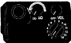
RESET THE SQUELCH KNOB to the Code Guard position (CG) to receive only the messages with the proper Code Guard value. During extended transmissions the squelch can be left open (off the detent) until the exchange has ended.
