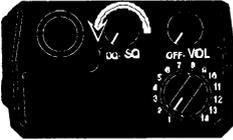
SET CODE GUARD MODE by turning the Squelch knob completely counterclockwise, past the detent to the CG position. A message will be heard only when the proper Code Guard value is received.
