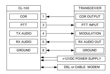
**Transceiver Interface** In this configuration the CL-100 is connected between a transceiver and a DSL or CABLE modem.
