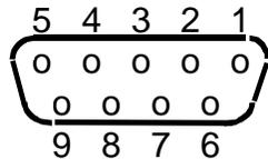
**J1-1 DC POWER INPUT-** Power input to the TP-3200 should be 12.6 VDC +/-20% regulated or unregulated obtained from the repeater power supply. If the AC wall transformer is used, connect the wire with the white stripe (+12VDC) to J1-1. Connect the other wire (ground) to J1-6.
