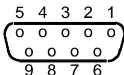
If you cannot communicate with the TP-3200 using your computer, check to make sure that the serial cable is wired properly. Make sure the cable you are using is a 'straight thru' cable. That is, pin 1 connects to pin 1, pin 2 connects to pin 2, and so on. Your computers serial port should be configured as a standard DTE device. The TP-3200 is configured as a standard DCE device. If you are still having trouble, try using a 'null modem cable adapter'.
