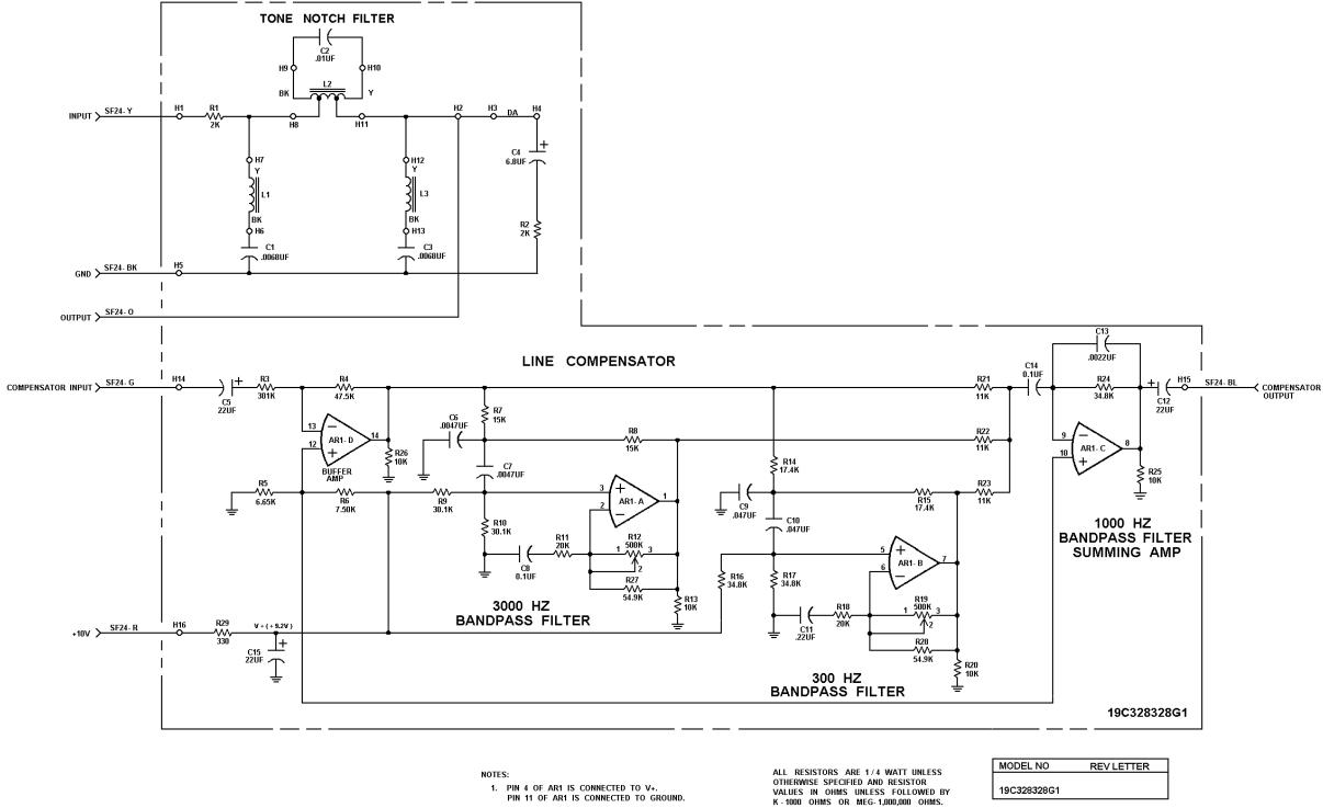
A - 1000 OHMS OR MEG-1,000,000 OHMS. CAPACITOR VALUES IN PICOFARRADS (EQUAL TO MICROMICROFARRADS) UNLESS FOLLOWED BY UF-MICROFARRADS. INDUCTANCE VALUES IN MICROHENRYS UNLESS FOLLOWED BY MH-MILLIHENRYS OR H-HENRYS.
