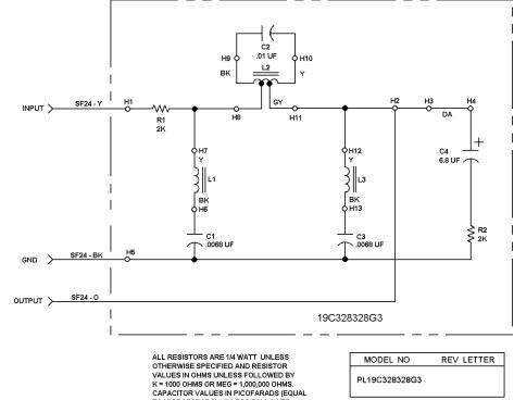
CAPACITOR VALUES IN PICOFARADS (EQUAL TO MICROFARADS) UNLESS FOLLOWED BY UF = MICROFARADS. INDUCTANCE VALUES IN MICROHENRYS UNLESS FOLLOWED BY MH = MILLIHENRYS OR H = HENRYS.
