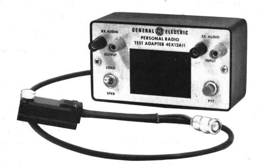
General Electric Test Adaptor, Model 4EX12All, provides audio connections for servicing transmit and receive circuits in MPR personal radios. A cable connected to the UDC connector of the MPR radio connects the audio to audio jacks on the front panel of the Test Adaptor. The audio jacks permit using standard dual-banana plugs for making connections to external test equipment.
