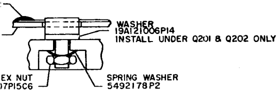
VIEW D TYP MOUNTING FOR Q201-Q203 ENLARGED
