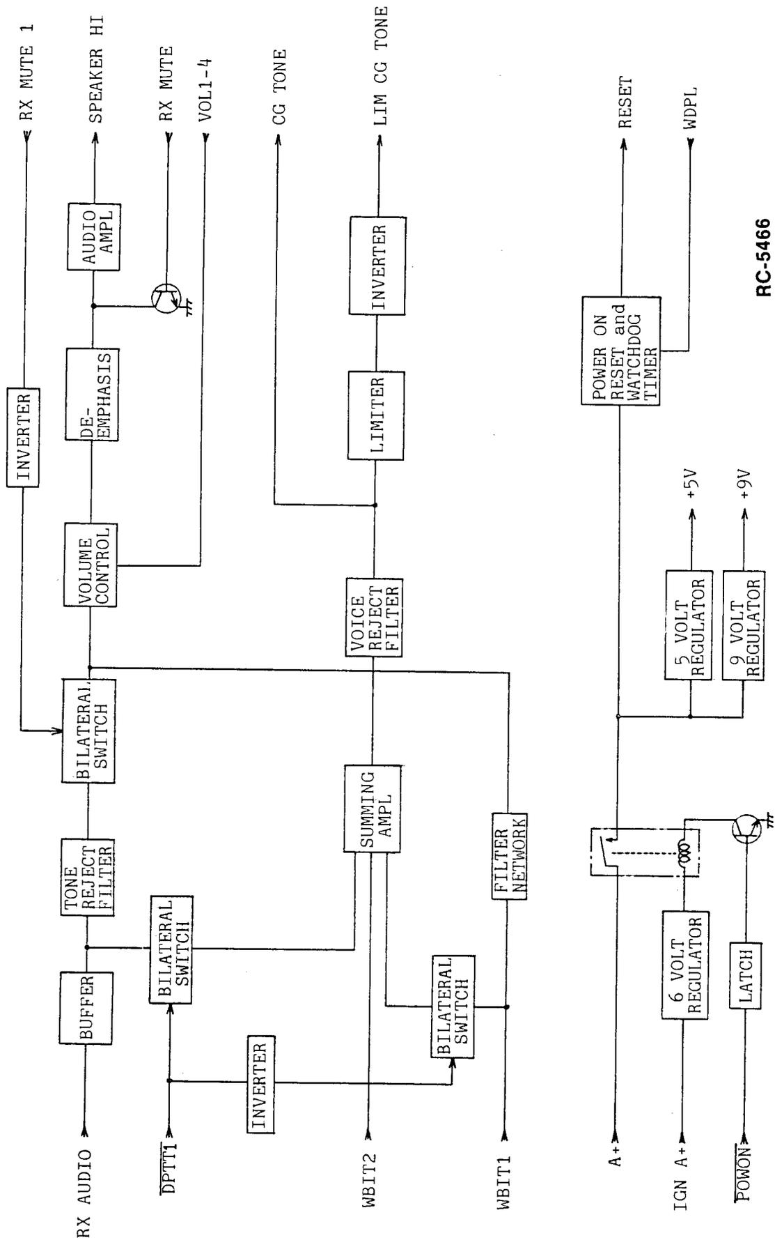
Figure 3 - System Control 2 Block Diagram
