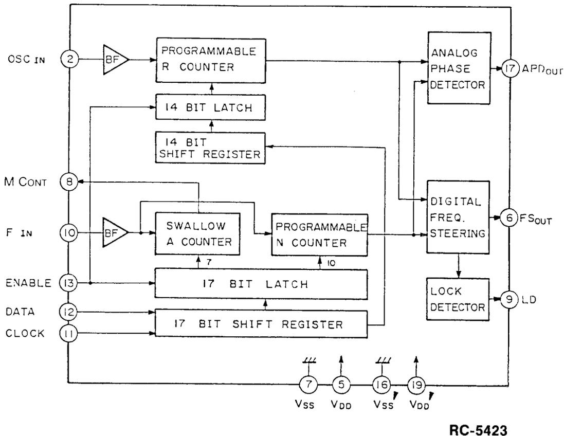
Figure 5 - Synthesizer IC201
