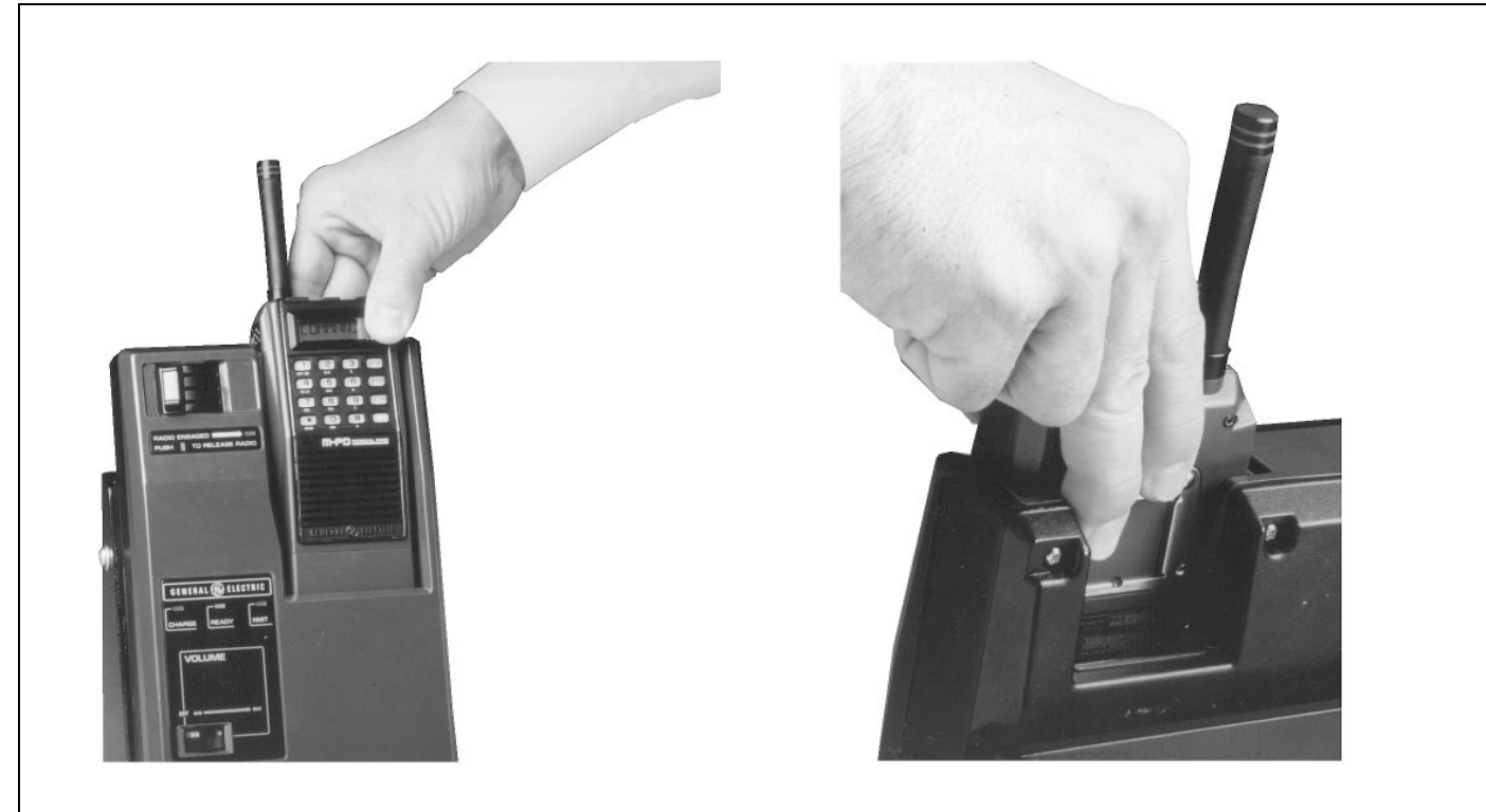
Figure 2 - Inserting and Removing Portable Radio Unit
