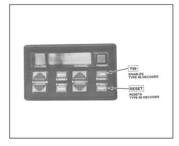
If the Type 99 Option is present, individual selective calling is possible. Press the T99 button to enable the decoder option. (Scan must be off). The LCD will show "OPT" in the upper center portion of the display. When a call is received, an alert tone will be heard and the OPT indicator will flash continuously. After receiving the call, press the RESET button to reset the decoder for the Next call. The OPT indicator will stop flashing.
