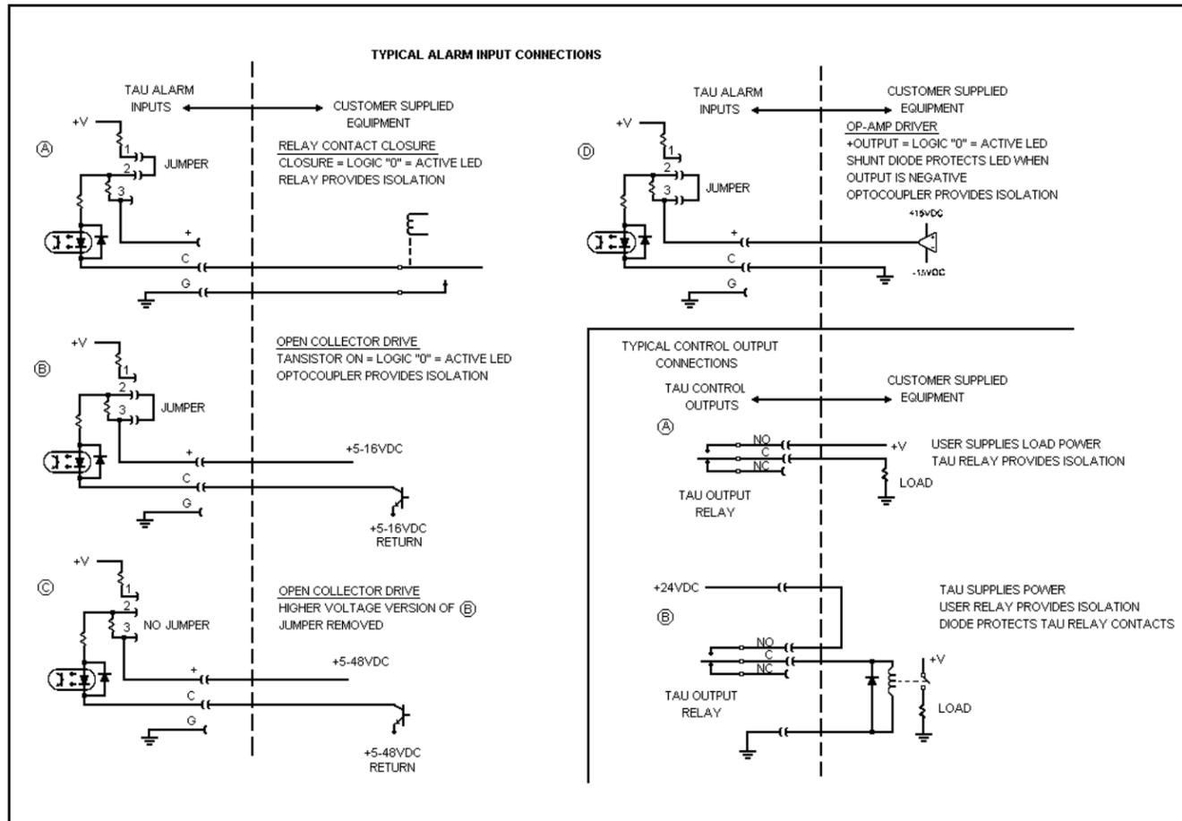
Figure 5 - Typical Alarm/Control Hookups
