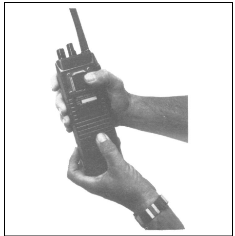
Figure 5 - Removing the Battery Pack
