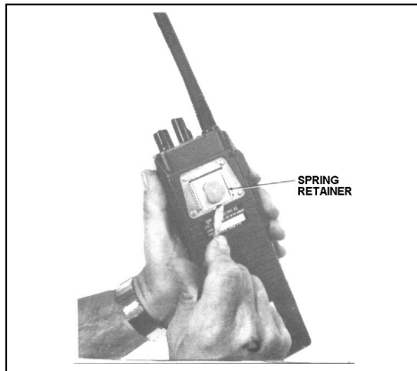
Figure 6 - Swivel Mount Removal and Replacement
