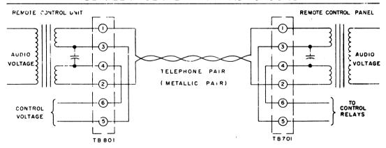
METHOD 3 - SINGLE TELEPHONE PAIR WITH CONTROL SIMPLEXED LINE TO LINE
