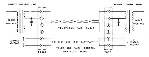
METHOD I - SEPARATE CONTROL AND AUDIO PAIRS
