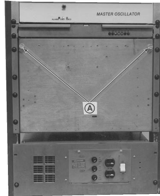
Figure 3 - Access To Knobs Securing Door
