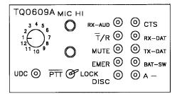
METERING JACKS ARE TIP JACKS MIC HI JACKS ARE 3/4" GR JACKS PTT SWITCH IS SPDT WITH CENTER OFF UDC SW. IS MIN. OF 10 POS.
