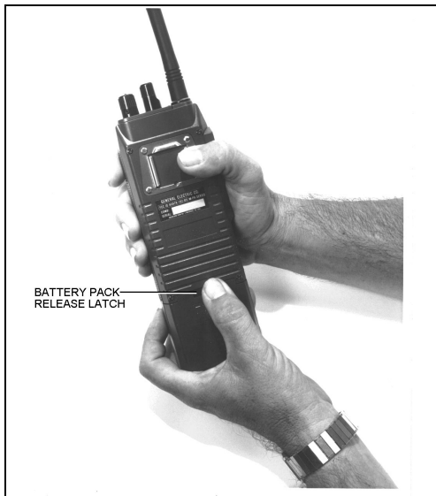
Figure 9 - Removing The Battery Pack
