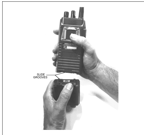
Figure 3 - Installing the Battery Pack
