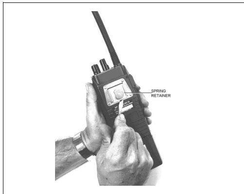
Figure 5 - Swivel Mount Removal and Replacement
