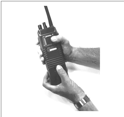
Figure 4 - Removing the Battery Pack
