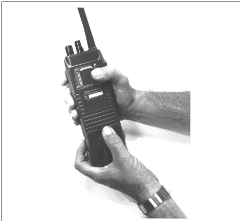
Figure 4 - Removing the Battery Pack
