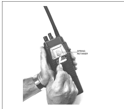
Figure 5 - Swivel Mount Removal and Replacement
