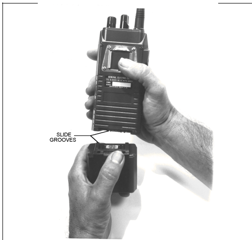
Figure 4 - Installing the Battery Pack
