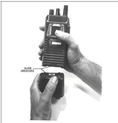
Figure 4 - Installing the Battery Pack
