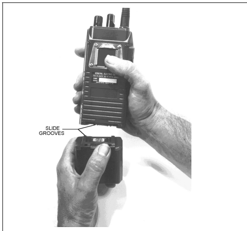
Figure 7 - Installing the Battery Pack
