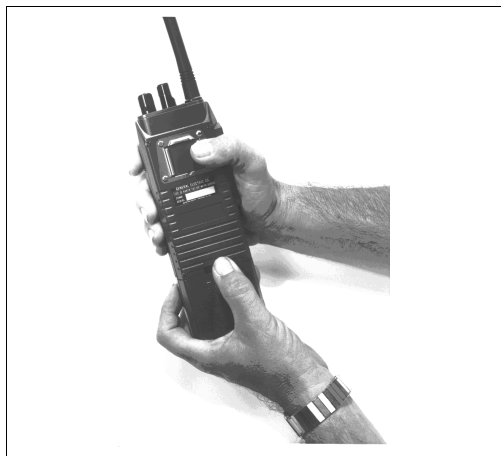
Figure 8 - Removing the Battery Pack
