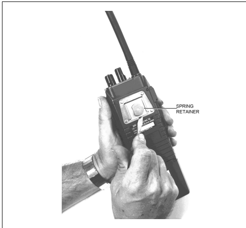
Figure 9 - Swivel Mount Removal and Replacement
