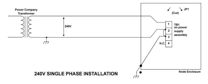
\* IT IS RECOMMENDED THAT THE NODE BE GROUNDED PER THE NEC (National Electric Code)
