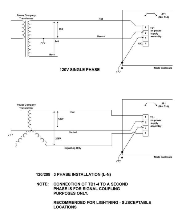
\* IT IS RECOMMENDED THAT THE NODE BE GROUNDED PER THE NEC (National Electric Code)
