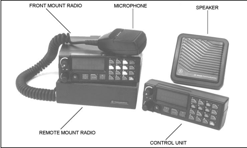
Figure 1 - Orion Mobile Radio Components And Mounting Hardware
