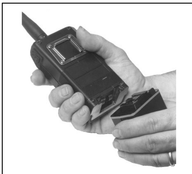
Figure 4 - Installing the Battery Pack
