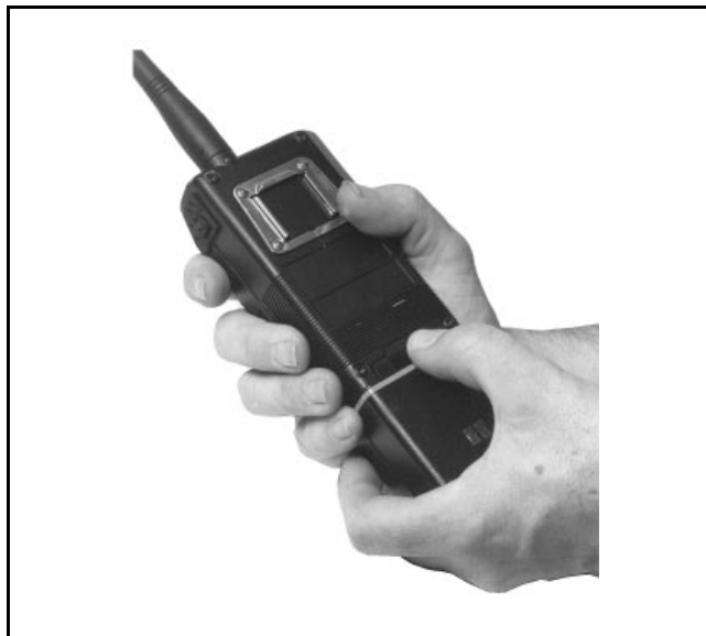
Figure 3 - Removing the Battery Pack
