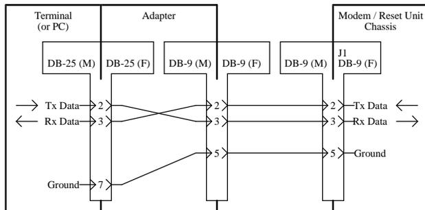
Figure 4 - Data Interface Adapter Connections
