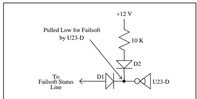
Figure 6 - GETC Failsoft Enable Circuit
