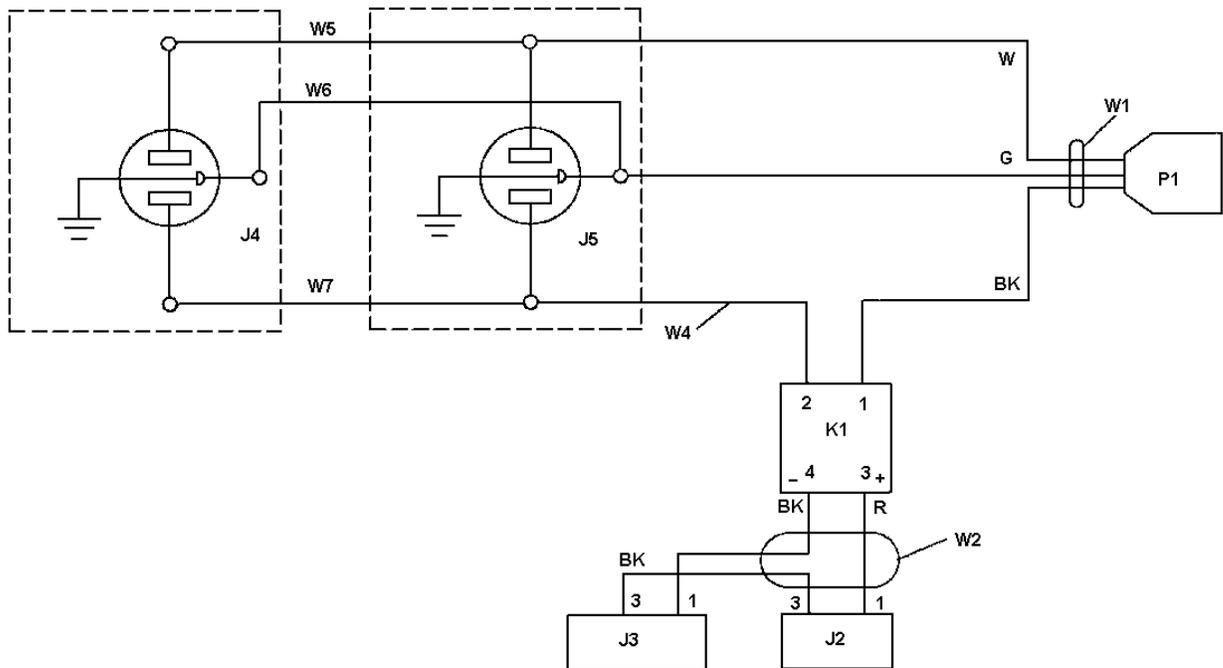
AC Relay Panel Interconnection Diagram
