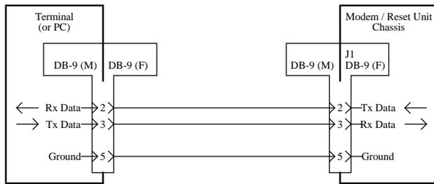
Figure 3 - Data Interface Cable Connections
