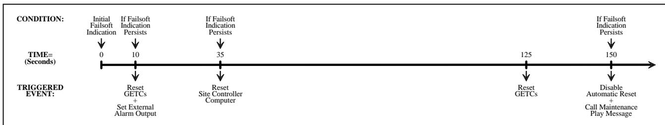
Figure 1 - Simplified Automatic Reset Cycle
