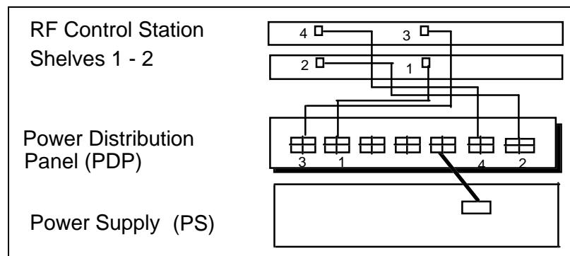
Figure 9 - Power Cabling of RF Control Stations
