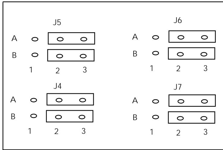
Figure 7 - Jumping SCI-232 for DTE
