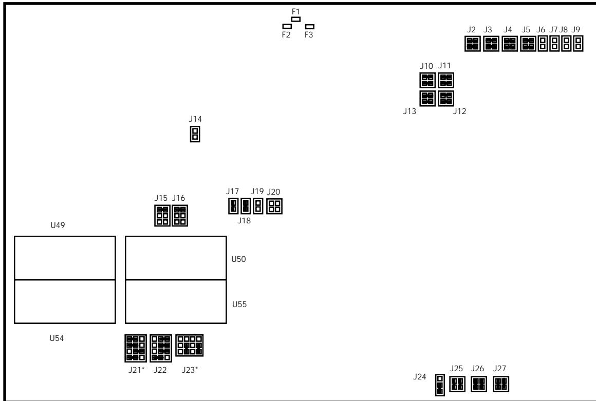
Figure 6 - VCOM24 Board Jumper Settings, Fuses, and Sockets
