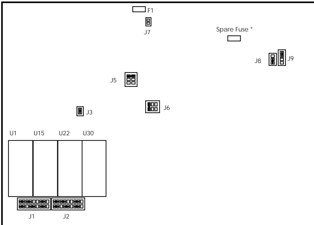
Figure 5 - MVME147 Board Jumper Settings, Fuses, and Sockets
