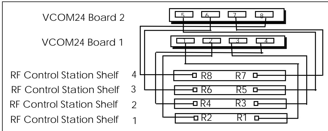
Figure 8 - Interconnection between RF Control Stations and VCOM24 Serial Ports
