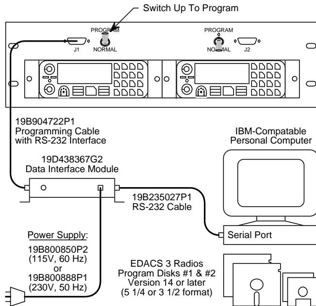
Figure 10 - Programming Setup
