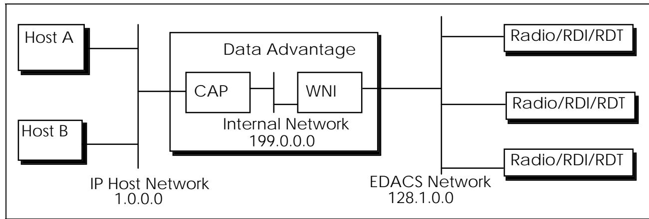
Figure 3 - An IP Host internet with Network Addresses assigned
