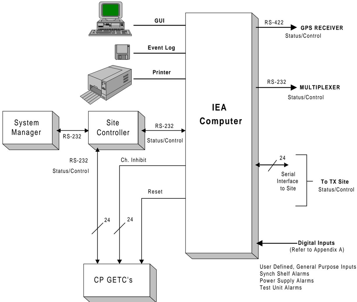
**Figure 1 - IEA System Block Diagram (Simulcast Control Point)**
