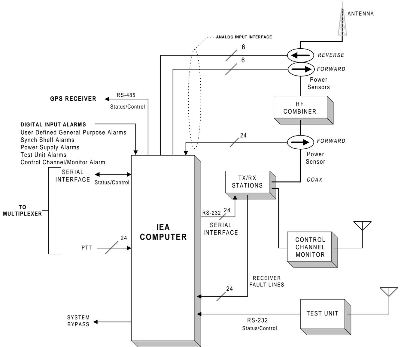
Figure 2 - IEA System Block Diagram (Simulcast Transmit Site)
