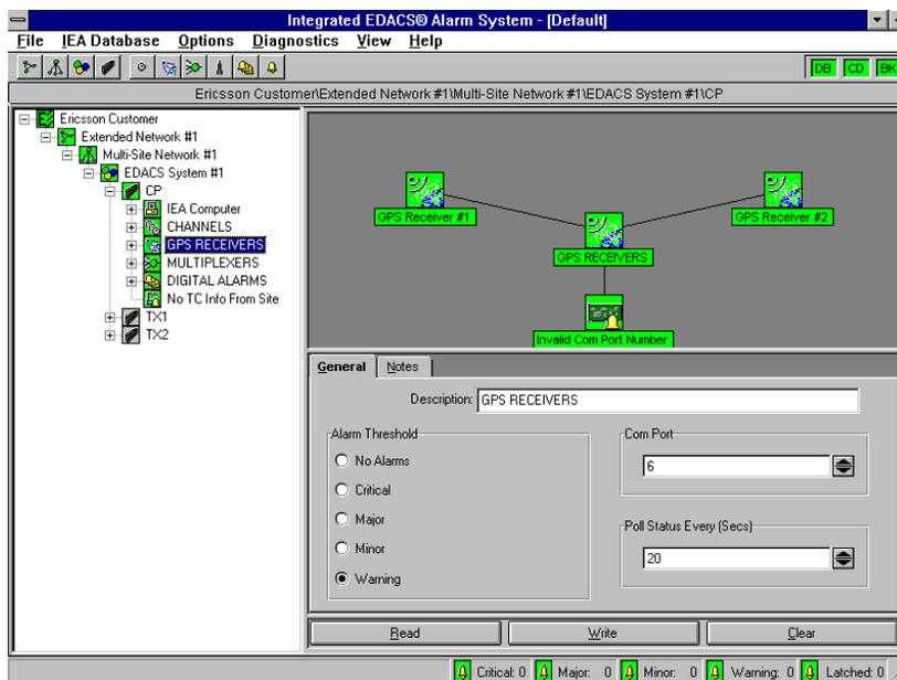
Figure 76 - EDACS Site with 2 GPS Receivers
