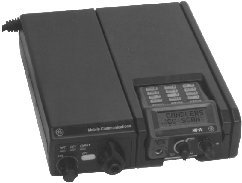
Figure 2 - Charger With M-RK II Personal Radio Inserted (Antenna Removed For Photo Only).
