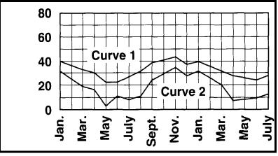
Figure 2 – Soil Resistivity by Seasonal Variation (With an electrode of <sup>3</sup>/<sub>4</sub> inch pipe in rocky clay soil. Depth of the electrode in earth is 3 ft for curve 1, and 10 ft for curve 2.)
