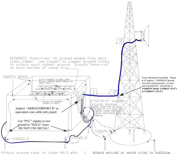
Attach ground rods to inside HALO with Smooth bends and using # 2 solid copper. Make all bends flow in the same direction at all four corners. Do not allow ground wire to contact other metal conduits 2 or cabinets between HALD and outside 3 ground rod(s).
