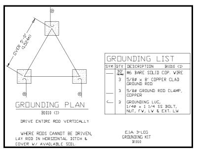
Figure A-1 3 Leg Tower Grounding Kit
