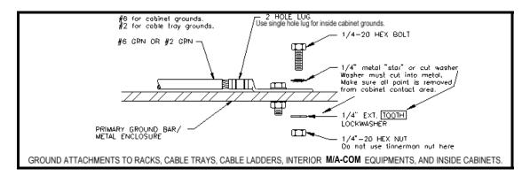
Figure 21 - Ground Attachment Methodology
