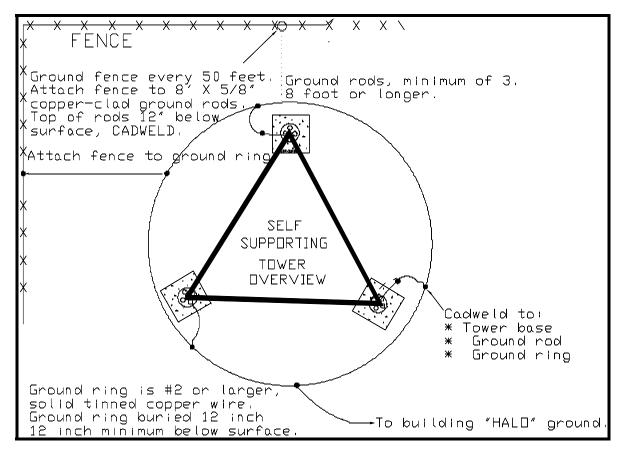
Figure 11 - Typical Transmit/Receive Site
