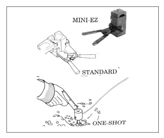
Figure 15 - Examples of the Tools Used to Make Exothermic Welds
