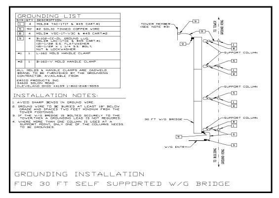
Figure A-8 30' Self-Supported W/G Bridge Grounding Kit
