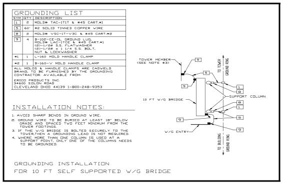
Figure A-6 10' Self-Supported W/G Bridge Grounding Kit
