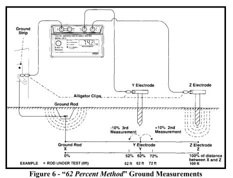
Figure 6 shows ground measurements made using the AEMC 4610, and AEMC 4500 (Commonly referred to as the "62 percent method."
