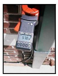
Figure 5 - Ground Measurement Using the AEMC Model 3730
