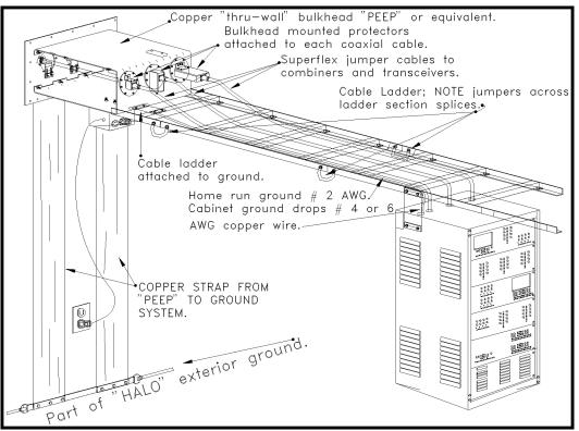
Figure 20 - Ground Attachments in Installation
