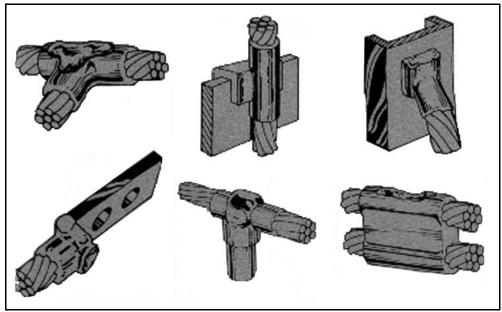
Figure 14 - Typical "Exothermic" Welds Made Using the Cadweld Method.
