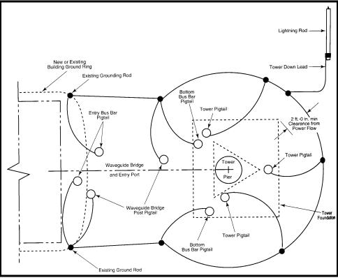
Figure 8 - Tower Halo Ground Ring
