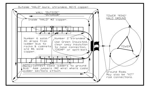
Figure 9 – In-Building Halo Ground Ring
