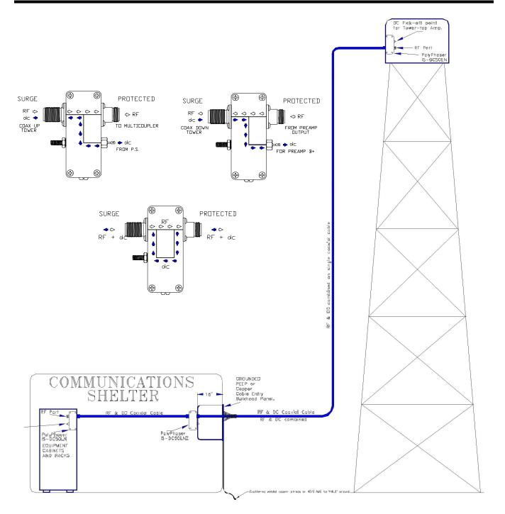
Figure 10 - Tower - Top Amplifier & DC Power Insert/Pick-Off Connections
