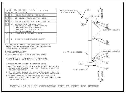
Figure A-7 20' Ice Bridge Grounding Kit
