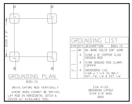
Figure A-3 Four Leg Tower Grounding Kit
