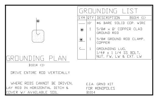
Figure A-4 Monopole Tower Grounding Kit
