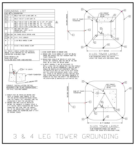
Figure A-9 3 and 4 Leg Tower Grounding Kit
