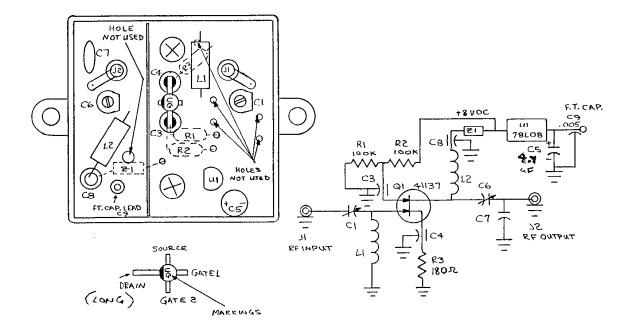
LNG-28 and LNG-50 Receiver Preamps, Schematic and Component Location Diagrams
