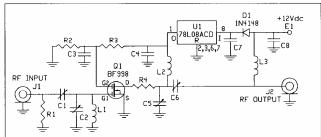
Figure 1. LNK Preamp, Parts Location and Schematic Diagrams
