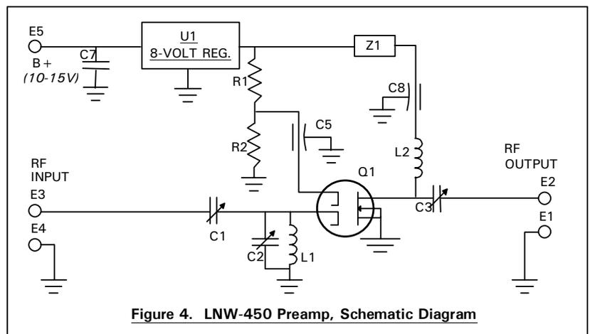
Figure 4. LNw-450 Preamp, Schematic Diagram
