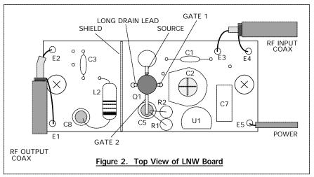
though protection is provided in the LNW in the form of a voltage regulator ic, avoid such conditions as a matter of principle. Care should be taken especially to install a reverse diode across any inductive devices, such as relays, on the same B+line to absorb transients.
