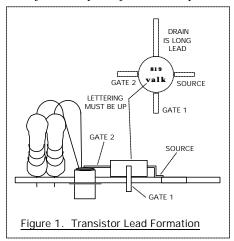
with solder as long as the three leads are all soldered at the top.
