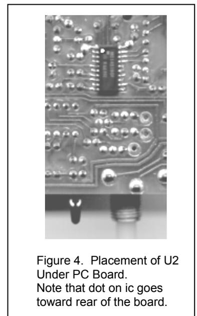
Figure 4. Placement of U2 Under PC Board. Note that dot on ic goes toward rear of the board.
