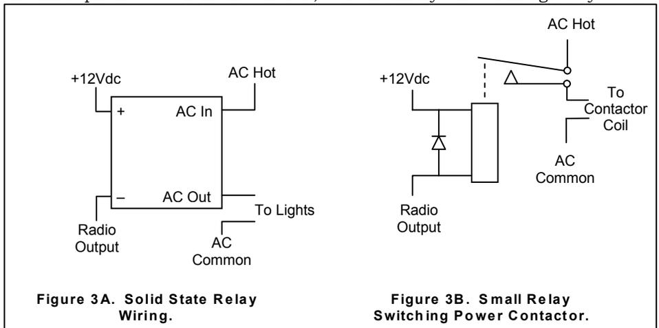
Figure 3A. Solid State Relay Wiring.
