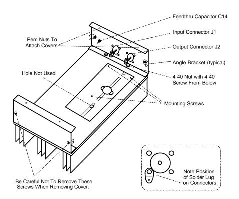
Figure 1. Bottom View of Heatsink and End Plates
