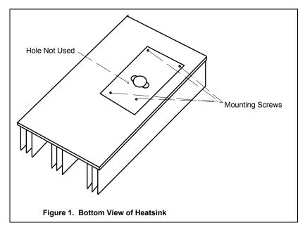
and note that the collector lead is the narrow one (see component location diagram). The collector lead should face the right-hand side (toward connectors). Apply a small amount of heatsink compound to the bottom surface of the transistor, and set it in place through the cutout in the board.
