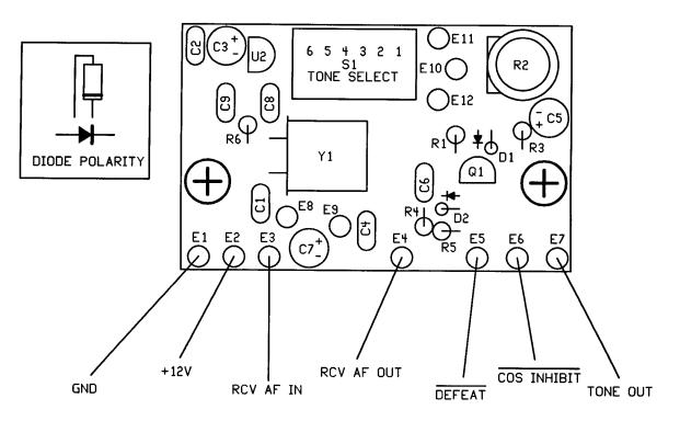
Figure 2. TD-5 CTCSS Encoder/Decoder, Parts Layout Diagram.
