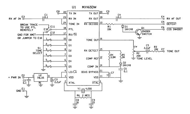
Figure 3. TD-5 CTCSS Encoder/Decoder, Schematic Diagram.
