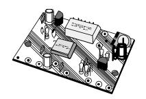
**CAUTION.** The TD-5 contains static sensitive ic's, which require normal static prevention techniques when handling to avoid damage. Wearing a grounded wrist strap is a prudent practice. For wired units, do not remove the unit from its protective package until ready to install. For kits, do not open package with semiconductors until ready to install on board.
