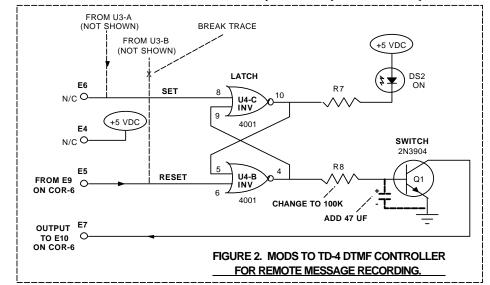
board from U3-B to U4-B as shown. Then, change R8 on the TD-4 to 100K, and add a  $47\mu F$  electrolytic capacitor from the base of Q1 to ground, as shown.
