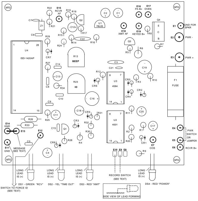
FIGURE 4. COR-6 REPEATER CONTROLLER MODULE, COMPONENT LOCATION DIAGRAM
