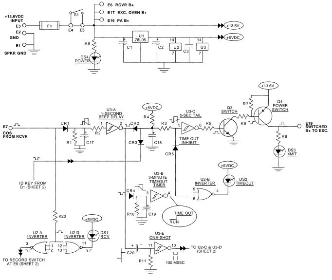
FIGURE 5A. COR-6 REPEATER CONTROLLER MODULE, SCHEMATIC DIAGRAM (SHEET 1)
