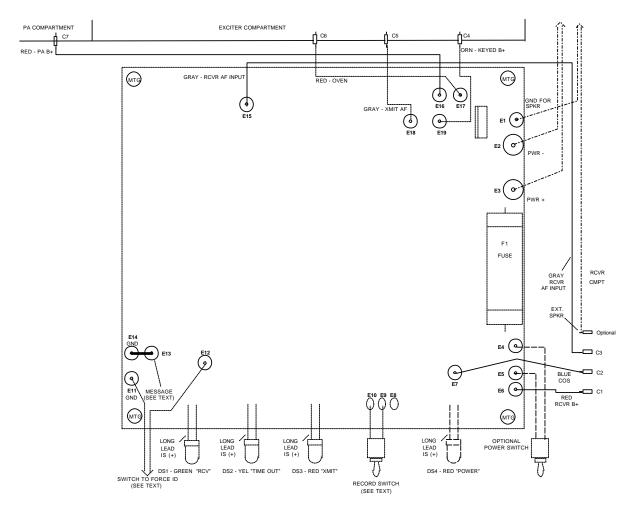
FIGURE 3. COR-6 REPEATER CONTROLLER MODULE REP-200C REPEATER INTERCONNECTIONS DIAGRAM
