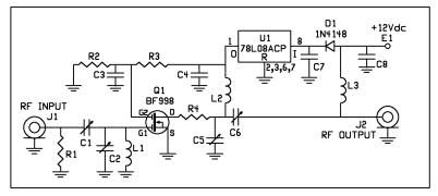
Figure 1. LNK Preamp, Top & Bottom Parts Location and Schematic Diagrams
