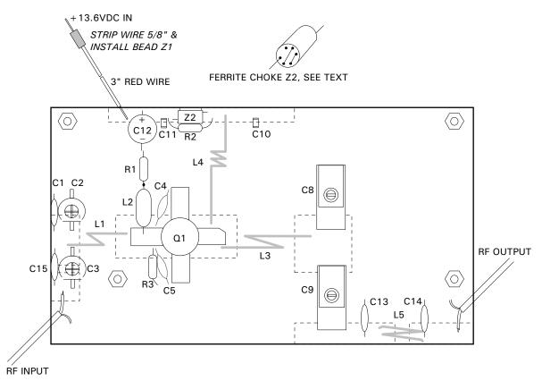
Figure 2. LPA 2-25R, Component Location Diagram
