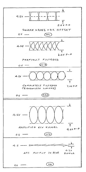
Figure 1. Waveforms at Major Circuit Points
