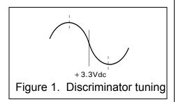
h. Connect signal generator to J1 using a coax cable with RCA plug. Adjust signal generator to exact channel frequency, and turn output level up fairly high (about  $1000\mu$ V). Adjust frequency trimmer in TCXO to net the crystal to channel frequency, indicated by +3.3Vdc at test point TP-6.
