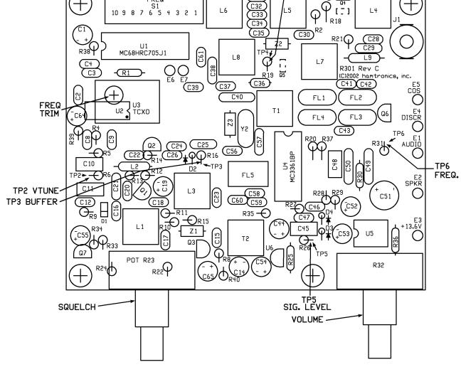
Figure 2. R301 VHF FM Receiver Rev C, Component Locations
