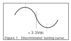
h. Connect signal generator to J1 using a coax cable with RCA plug. Adjust signal generator to exact channel frequency, and turn output level up fairly high (about  $1000\mu$ V). Adjust frequency trimmer in TCXO to net the crystal to channel frequency, indicated by +3.3Vdc at E4.
