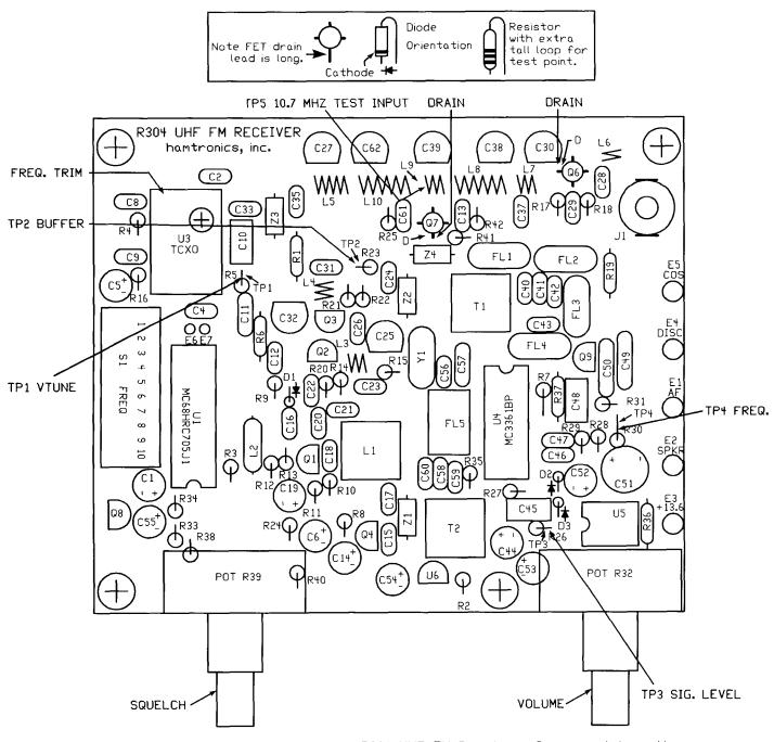
Figure 2. R304 UHF FM Receiver, Component Locations
