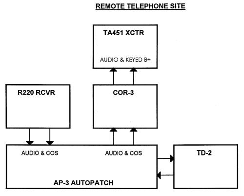
This is a tentative layout of how to link an REP-200 Repeater with an autopatch at a remote site. Set beep delay on COR-3 to about 1/2 second and tail time to zero so autopatch can turn around quickly between transmit and receive.
