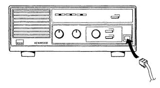
3 Connect the KPT-50 cable with the 8-pin connector to the matching connector facing upward inside the unit immediately behind the front panel.
