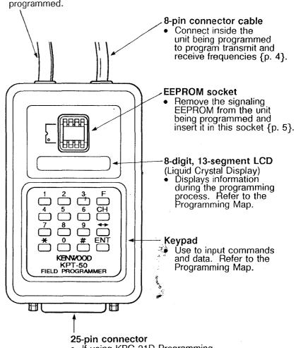
If using KPG-21D Programming Software, connect the interface cable from a computer to this connector. Refer to the KPG-21D Instruction Manual.
