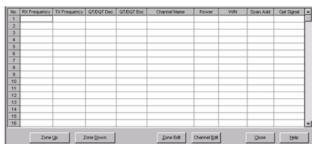
Figure 6-2 Zone Information Window (Conventional Group)
