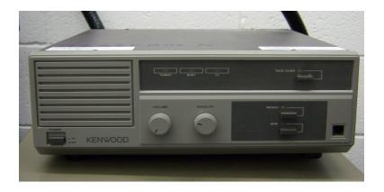
This is my experience in adding an ID-O-Matic II to a Kenwood TKR-720 VHF Repeater for 2-meter use. The same steps can be used to modify a TKR-820 UHF Repeater for 70-centimeter use.
